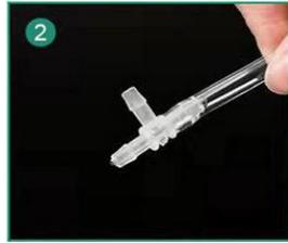
2. Connect the tubing to the branch lines.
