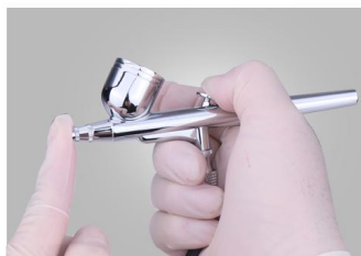
2. With the airbrush working, place your index finger cover the airbrush nozzle to block airflow.
