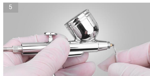
Unscrew the airbrush nozzle.
