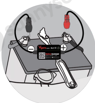
Connecting the product to the battery
