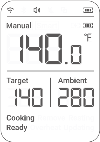
When it reaches 140°F the cooking is complete (the Ready icon lights up and alarms)
