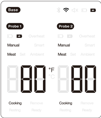
The probe is not charging correctly: the charging icon flashes and the buzzer keeps alarming. See Troubleshooting
