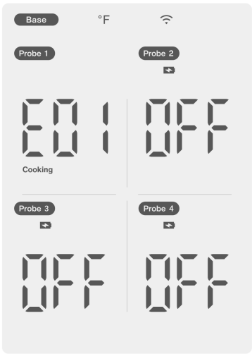
Probe malfunction, error code EXX reported
