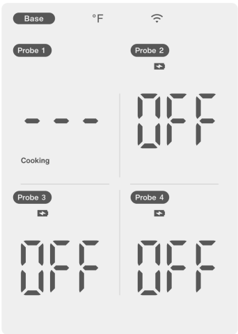
Probe 1 is disconnected
