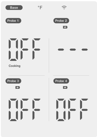
Probe 2 is disconnected
